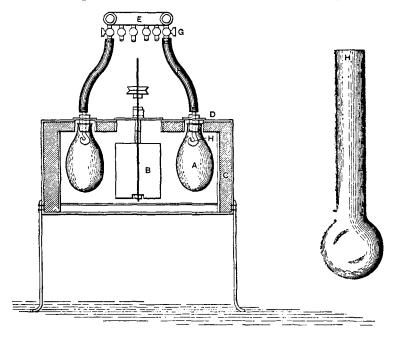
content ranges from 150 to 200 cc. It is closed with a rubber stopper carrying a water trap bulb, H H¹, arranged in such a way that the vapor of water which condenses within the exhaust tube, instead of falling back into the flask, remains trapped in the water bulb. All the flasks in the oven are connected by means of a common connection, E, with a vacuum pump capable of producing a vacuum of from twenty-six to twenty-seven
